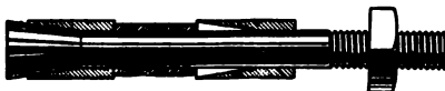
SECTIONAL VIEW SHOWING BOLT WITH PRIMARY EXPANSION SLEEVE, ONE IRON SPACING SLEEVE, AND ONE SECONDARY EXPANSIVE UNIT
